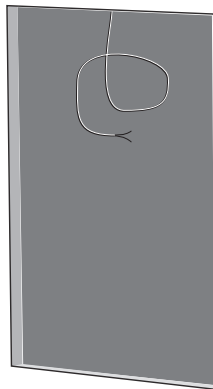
Fig. 3. Drywall Cutout with Speaker Cable
